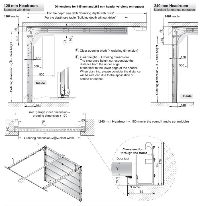
Please observe the following measurement details, to guarantee exact assembly and precise and reliable operation of the CarTeck sectional door.
